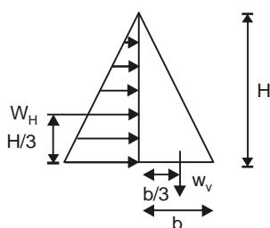
$$\sigma_{v \text{ toe}} = \frac{w_v}{b \times 1} + \frac{[W_v \times b / 6 - W_H \times H / 3]}{\frac{b^3 \times 1}{12}}$$
