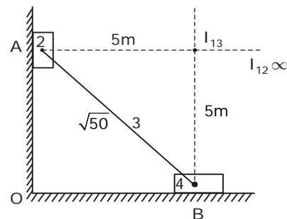
$$\begin{aligned} \text{Now } \omega_{AB} &= \frac{V_A}{I_{13}A} = \frac{V_B}{I_{13}B} \\ &= \frac{10}{5} = 2 \text{ rad/sec} \end{aligned}$$
