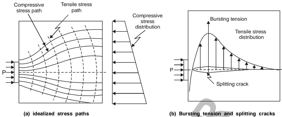
**End blocks of post-tensioned beams**
