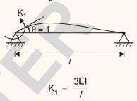
(ii) Stiffness of beam at near end when far end is fixed.
