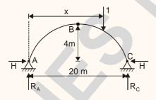
$\sum_{A} M_{C} = 0$   $R_{A} \times 20 - (20 - x) \times 1 = 0$   $R_{A} = \frac{20 - x}{20}$   $\sum_{B} M_{B} = 0$ , left of B.
