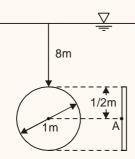
Total hydrostatic pressure force, $F = P_A.A$
